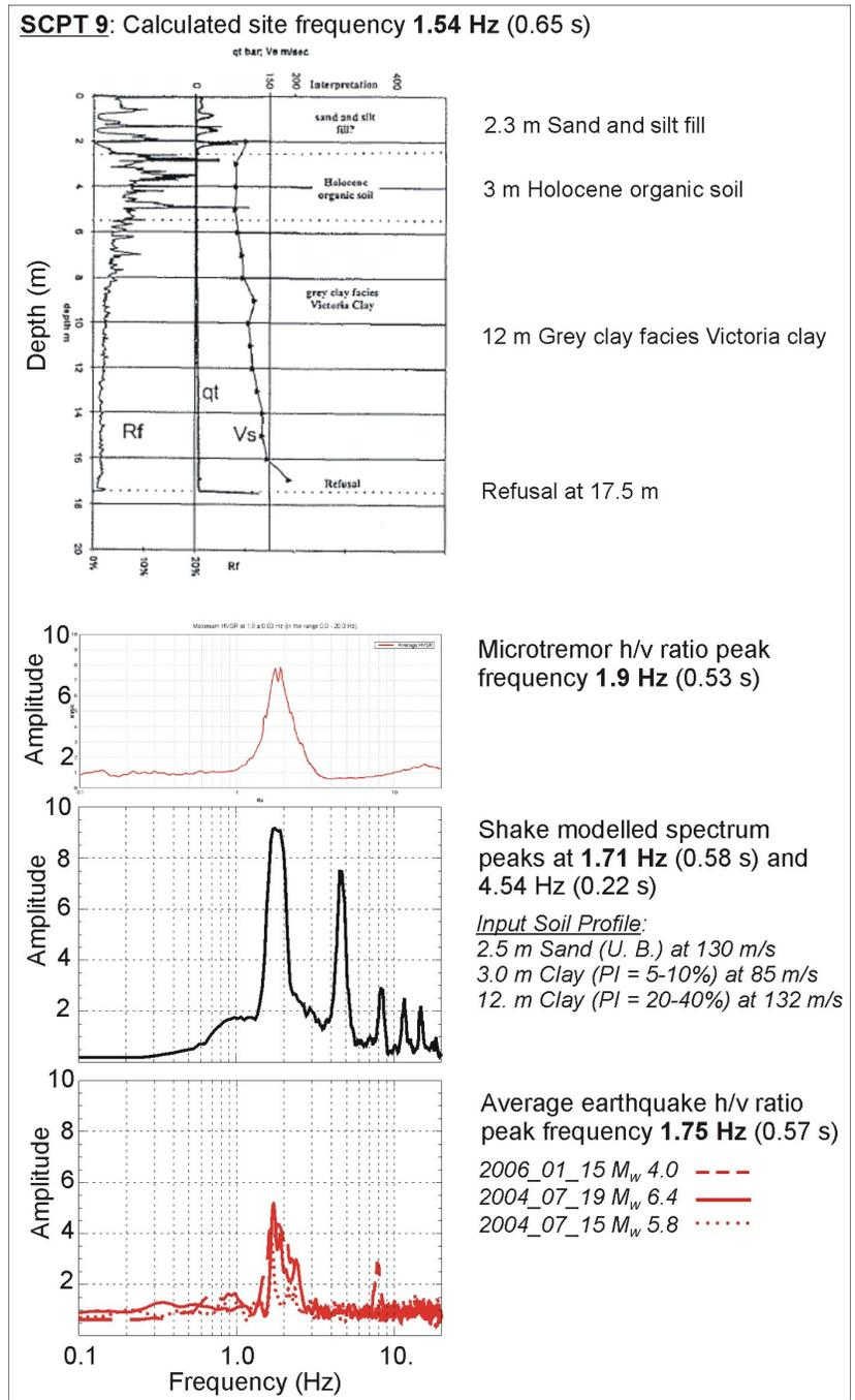
Figure 1. Comparison of peak frequency at SCPT 9 located in downtown Victoria from SCPT measurements, microtremor, SHAKE modelling, and weak earthquake motion. SCPT parameters:  $V_s$  = shear-wave velocity, qt = tip resistance, and Rf = friction ratio.
