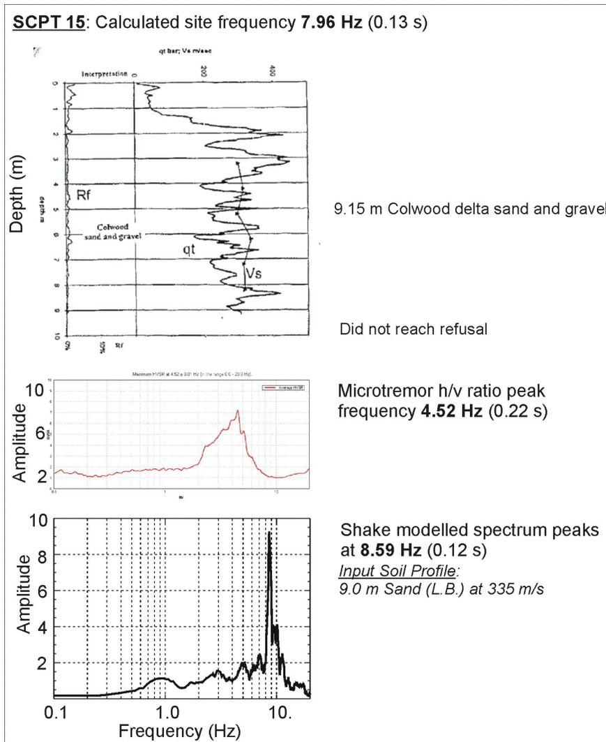
Figure 3. Comparison of peak frequency at SCPT 15 located on the Colwood sand and gravel delta from SCPT measurements, microtremor, and SHAKE modelling. SCPT parameters;  $V_s$  = shear-wave velocity, qt = tip resistance, and Rf = friction ratio.
