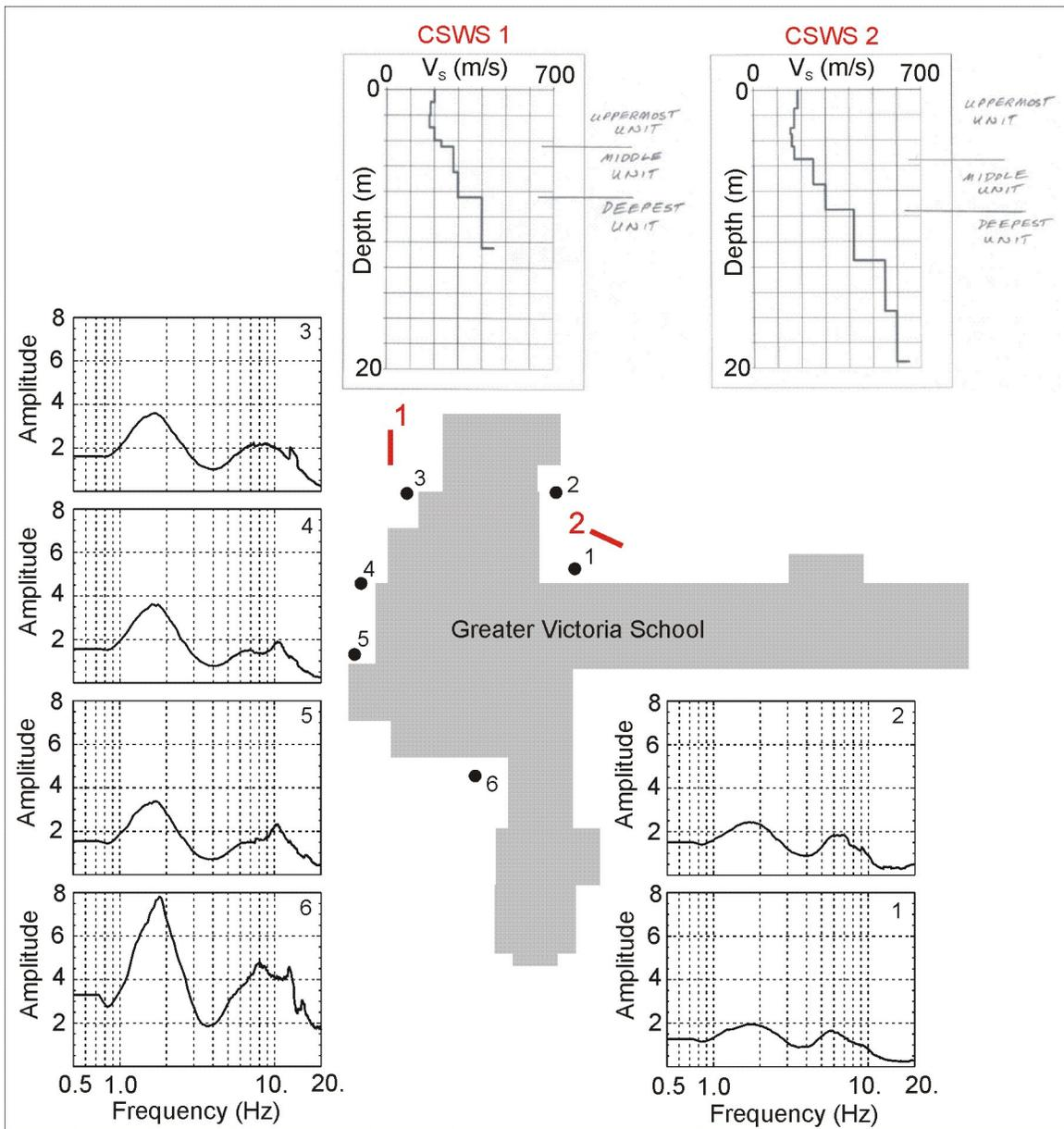
Figure 5. Comparison of peak frequency at CSWS test sites located atop of a glacial drumlinoid ridge of dense glacial Pleistocene material (till) from CSWS testing and microtremor measurements.
