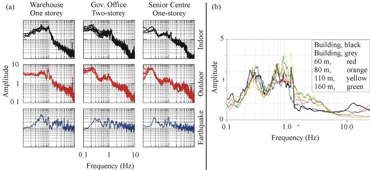
Figure 6. (a) Comparison of indoor and outdoor (within 50 m) microtremor and earthquake h/v spectral ratios at three strong-motion instrument locations in greater Vancouver demonstrate minor structural influence. Log-log plots. (b) Microtremor h/v spectral ratios 0 to 160 m distant of a 14-storey building are consistent. Log-linear plot.
